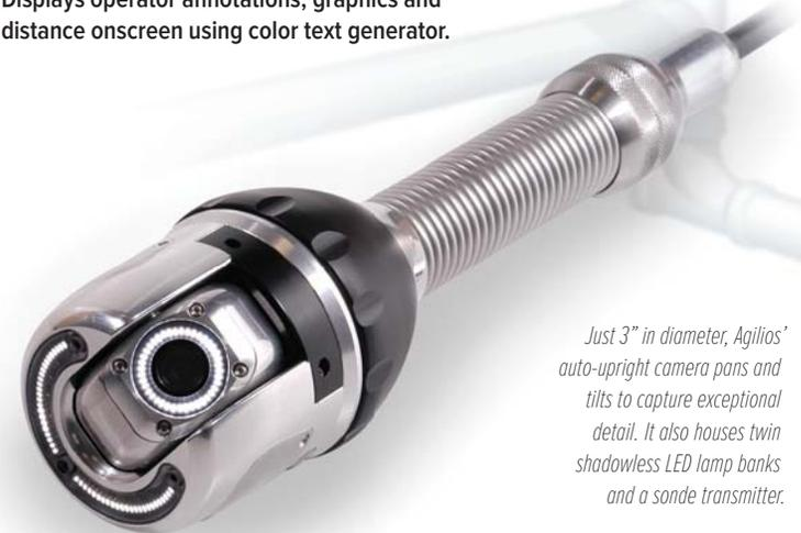
*Just 3" in diameter, Agilios' auto-upright camera pans and tilts to capture exceptional detail. It also houses twin shadowless LED lamp banks and a sonde transmitter.*
