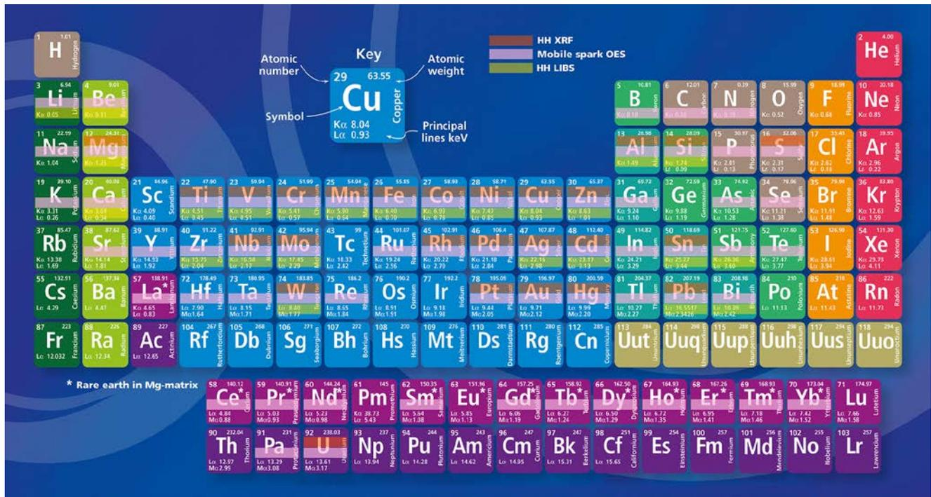
The periodic table displays which elements can be detected by which handheld / portable technology and thus facilitates the decision
