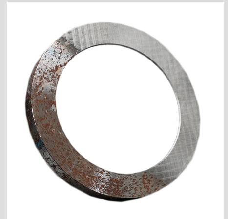
Corrosion Removal on Steel Ring
