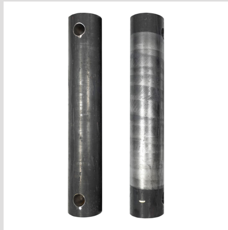
Laser Cleaning on Steel Pipe
